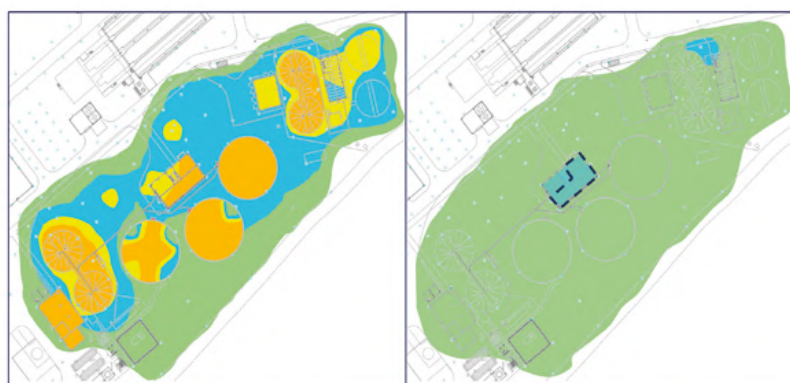
Figure 5. Concentrations of H 2 S (left) y relative humidity (right) in sludge line.
